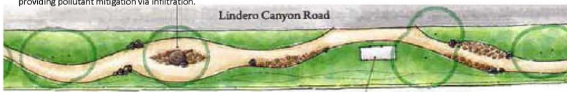
Figure 2: After Photo showing bio-swale eliminating runoff and providing pollutant mitigation via infiltration.
